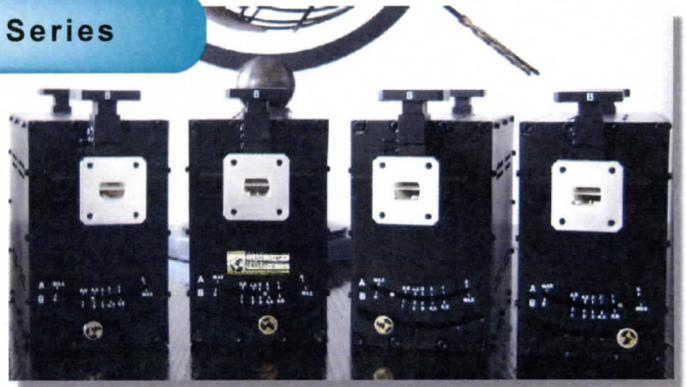
This is accomplished by varying manually the position of the polarizer under full power conditions which makes the **VPC** the most versatile combiner in the industry. If you wish to know more about the theory of operation of the VPC, refer to Canteq's **Application note No. 51**. Canteq produces very compact VPCs in most standard bands with exceptional performance. Our Ku and C band VPCs have been delivered to very demanding and prestigious customers and they are installed around the globe.
